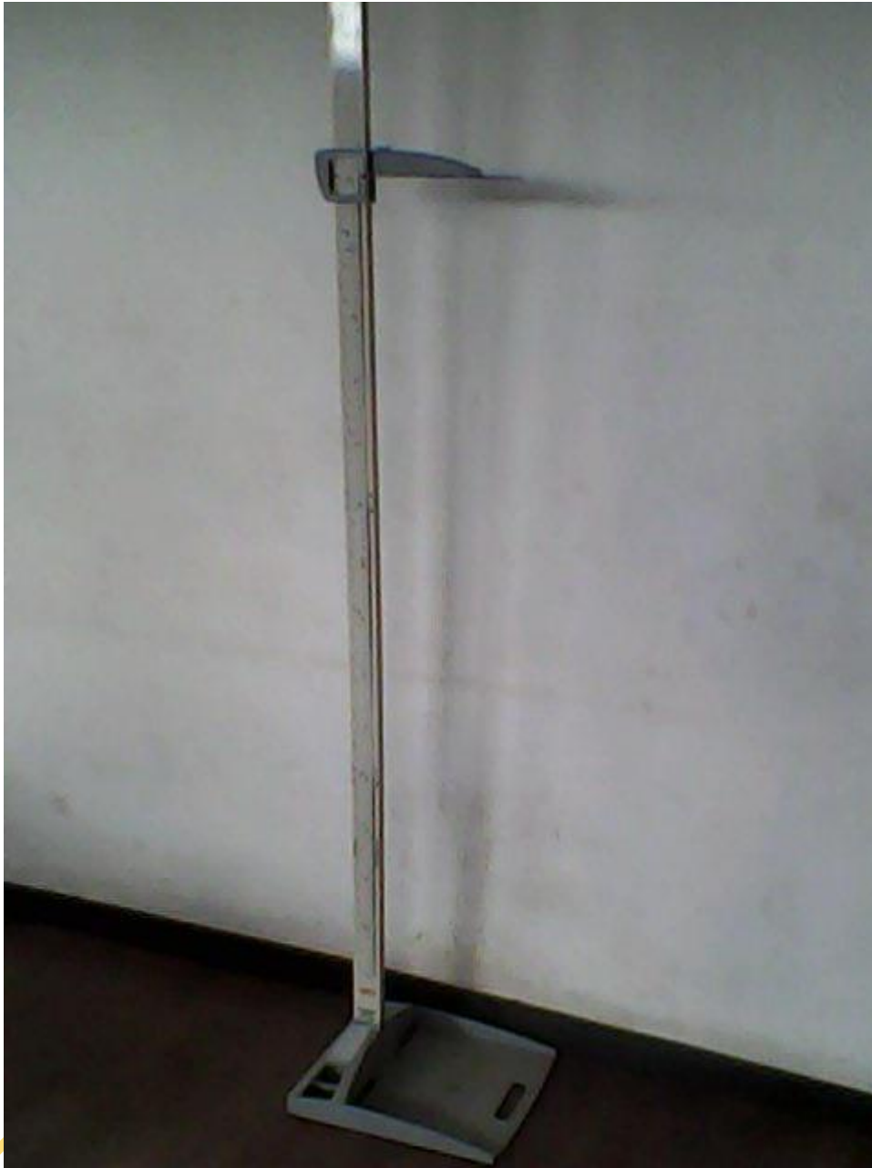
Plate 2. A height meter (SECA, Model 220) used to measure the heights of participants in centimeters.
